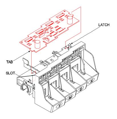
Figure 5-7. Carrier PCB Removal/Installation.
